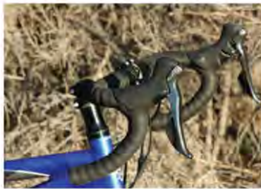
Above left: Barrell adjustors for the shifter cables are a nice touch on the Milano; Tiegra brifters and derailleurs give the captain full control of the team's future. Above right: Nothing much more personal and subjective than bicycle saddles, but our test team found the KHS padded road saddles to provided a nice enough ride. Alloy suspension post for the stoker is a nice – and appreciated – touch.
