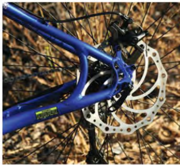
KHS spec'd Bengal MB700T, Mechanical Disc brakes with 203mm Rotors for the aluminum-framed Milano. Total weight is under 40 lbs.
