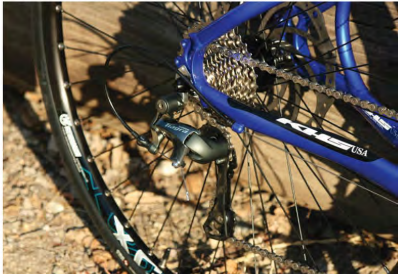
Above: Bright colors and eye-pleasing graphics are part of the package; KHS-branded chainrings have a precision-machined appearance, 50/39/30 ratios. Below: Shimano Tiagra derailleurs front and rear, 11-32 rear cassette provided easy, reliable shifts and range for our test team.
