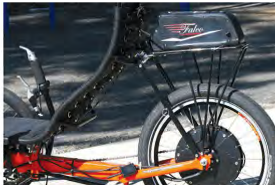
Above: Falco system was temporarily installed on a Greenspeed GT20 for reviewing the system. A more permanent installation would include a prettier job of routing the wires and accessories. Small black box contains circuitry and antenna for the ANT+ which allows the Falco's hub motor to communicate with the Android smart phone used during the test. Reviewer Zupke would prefer a lower mounting position for a permanent installation, freeing up the rack for other purposes. Below: The Falco's control display is within easy reach of the rider when mounted on the mirror stalk.
