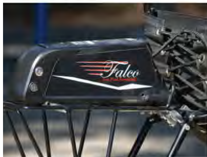
A range of battery sizes is available. More permanent installation options can be found. T-Cycle has a number of pre-fab mounts as well as assorted brackets and parts to make your own mount. The battery can be locked to the battery bracket with a keyed lock, above that is the on/off switch to the battery. Battery endurance depends on terrain, speed being maintained, overall load and tire selection
