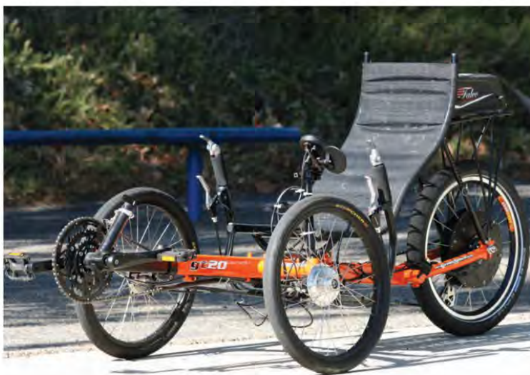
Our review setup from Falco was installed on a Greenspeed GT20. Falco supplied the motor laced to a Velocity Aeroheat wheel and Schwalbe 20 x 2.23 Big Apple tire. Components are available separately, but having the complete setup supplied ready to go make for an attractive package for either shops to install or home do-it-yourselfers.
