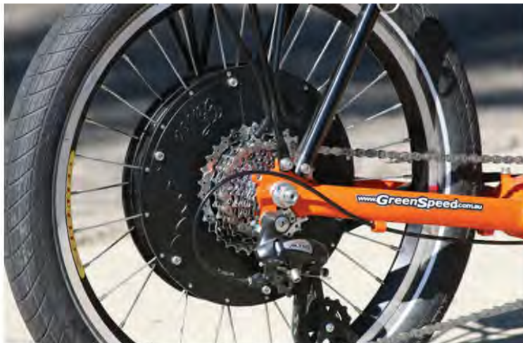
Falco's brushless electric motor is contained within the rear hub. Wheel size fitments include 700c, 29er, 650B, 26-inch, 24-inch, and 20-inch. Falco can build the wheel to your spec; motor options include 500 watt, 750 watt, and various battery capacity setups. Motor/battery combos are also available. The Falco system is compatible with 1/7/8/9 or 10-speed cassettes.
