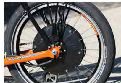
Power cable is routed through the bottom center portion on the left side of the hub. Hub needs to be 'clocked' into the correct position in the drop outs. An anti-torque tab keyed into the drop out keeps the center of the hub from spinning. The Falco motor is a five-phase, brushless design which causes no drag when the motor is switched off.
