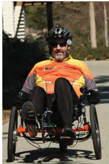
Electric assist is nice to have when facing long rides up steep hills. Back-pedaling downhill puts the system into 'regen' mode, wherein electricity is generated and sent to the battery. Regen also causes a decent amount of drag which can be utilized on long downhills to moderate speed rather than riding the brakes.
