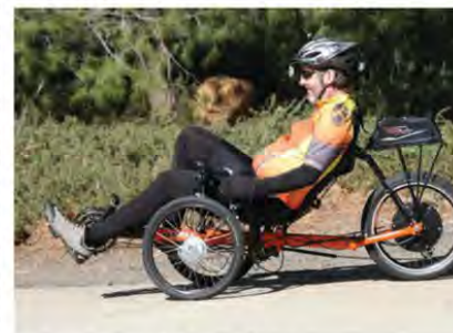
Above: Falco system was temporarily installed on a Greenspeed GT20 for reviewing the system. A more permanent installation would include a prettier job of routing the wires and accessories. Small black box contains circuitry and antenna for the ANT+ which allows the Falco's hub motor to communicate with the Android smart phone used during the test. Reviewer Zupke would prefer a lower mounting position for a permanent installation, freeing up the rack for other purposes. Below: The Falco's control display is within easy reach of the rider when mounted on the mirror stalk.
