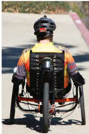
Electric assist is nice to have when facing long rides up steep hills. Back-pedaling downhill puts the system into 'regen' mode, wherein electricity is generated and sent to the battery. Regen also causes a decent amount of drag which can be utilized on long downhills to moderate speed rather than riding the brakes.
