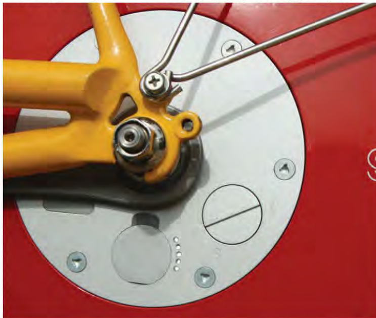
Battery charging port is on the left, five LED lights indicate level of charge, rotary switch to the right of that is the On/Off switch. (The On/Off icons are difficult to see in the photo.) The cap shown flipped up out of the way of the charger connection is held closed magnetically when charging is completed.
