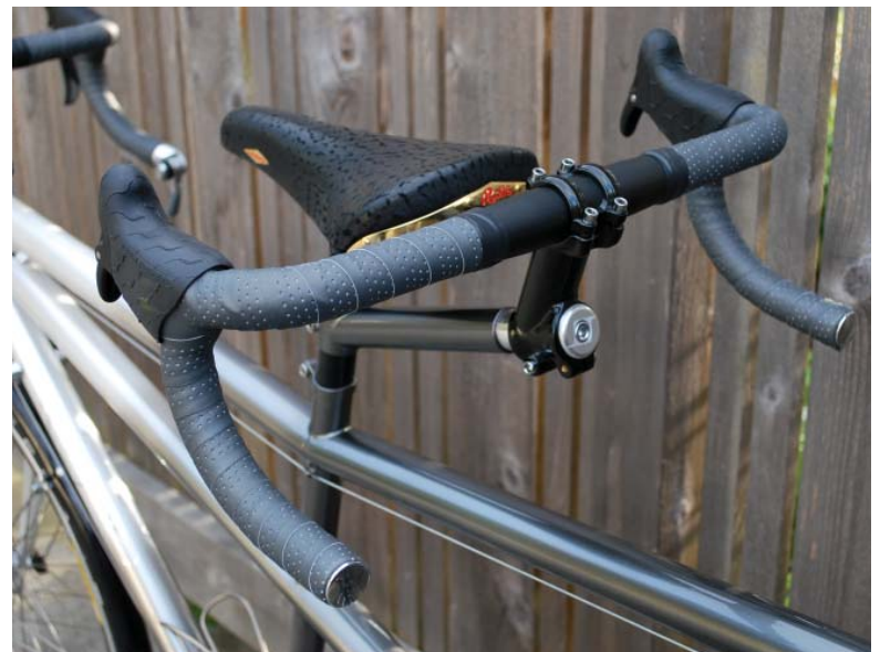
The stoker's cockpit features a special stem for a more upright riding position.
