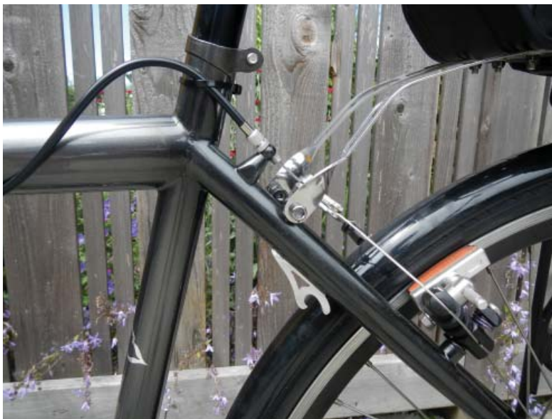
That's a bottle opener on the left seat stay, lots of attention to detail is evident.
