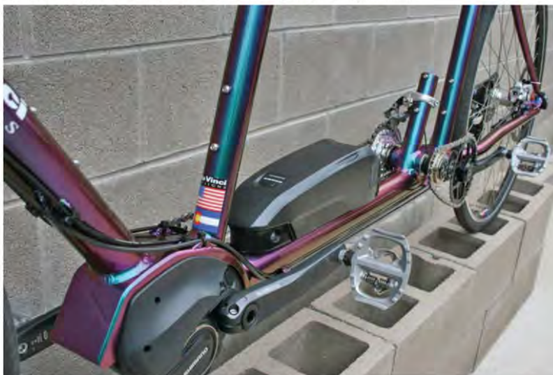
Above and below: Changes to the da Vinci ICS drive system required in order to incorporate the Shimano STEPS drive intuded moving the timing chain between the captain's and stoker's cranks for the left side to the right side. Battery is mounted on the boom tube just being the motor.
