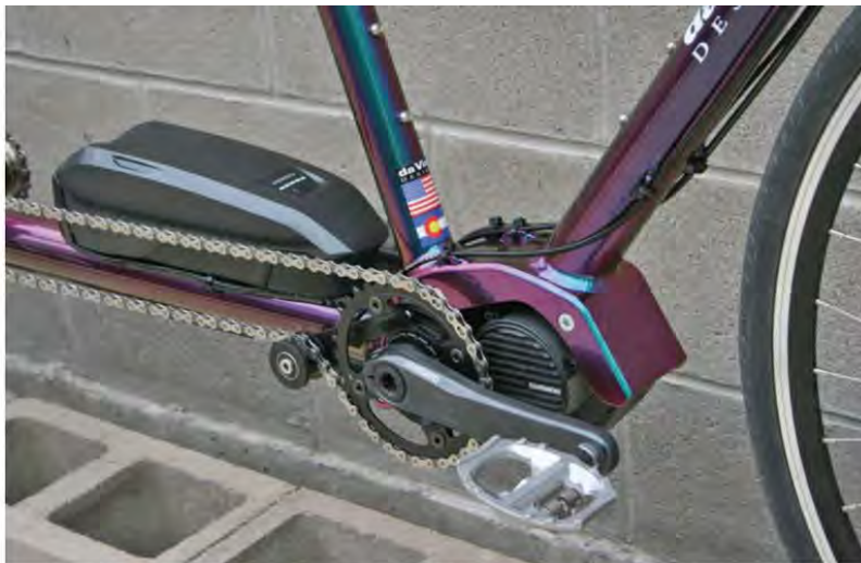
Above and below: Changes to the da Vinci ICS drive system required in order to incorporate the Shimano STEPS drive intuded moving the timing chain between the captain's and stoker's cranks for the left side to the right side. Battery is mounted on the boom tube just being the motor.
